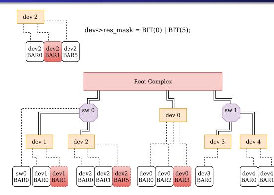
Reassignment may fail: blocked by fixed BARs, or not enough address space. A working layout must be restored.
