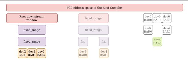
• A window set with the leftmost fixed BAR is assigned first, starting from the downstream root port;
