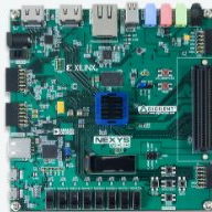
OpenPOWER Microwatt on Digilent Nexys Video
