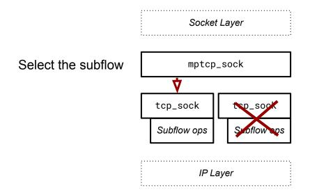
Sending of ACKs to signal options, e.g. REMOVE\_ADDR in a TCP ACK
