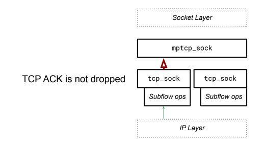
Reception of ACKs with signaling options, e.g. REMOVE\_ADDR in a TCP ACK
