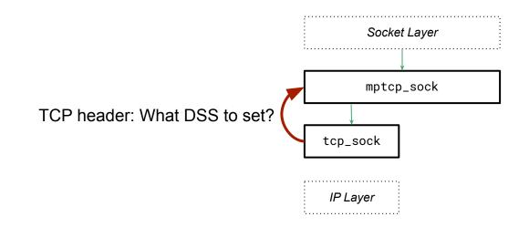
Sending of ACKs to signal options, e.g. REMOVE\_ADDR in a TCP ACK
