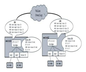
Fig 2. Bridging and Network virtualization
