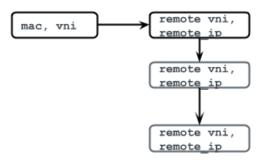
Fig 5. Current Vxlan FDB structure
