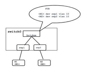
Fig1: Linux bridge on a switch bridging traffic between hosts
