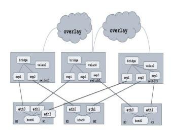
Fig 4: Multihoming with network overlay
