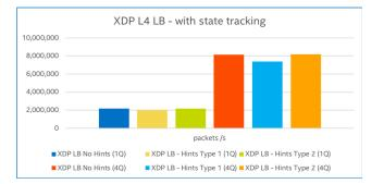
Figure 3: L4 LB with Hints, With State Tracking
