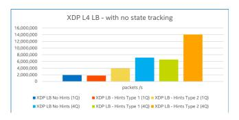
Figure 2: L4 LB with Hints, No State Tracking
