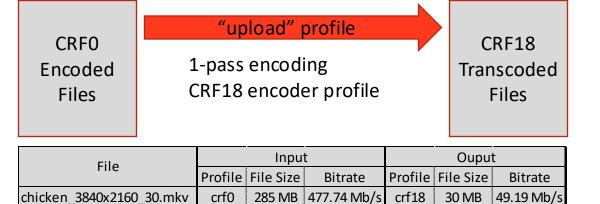
CRF (Constant Rate Factor): a single-pass encoding mode, you choose a quality target, and the encoder adjusts the bitrate to achieve that quality level.
