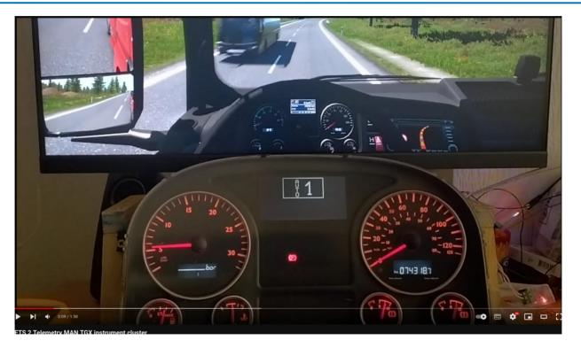
Connecting Euro Truck Simulator 2 to a real MAN TGX instrument cluster by using J1939 kernel stack
