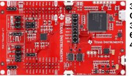
32-MHz Arm® Cortex®-M0+ MCU 32bit 64-KB flash, 4-KB SRAM
