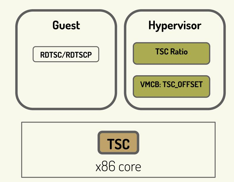
TSC Value (in guest) = (P0 frequency \* TSCRatio \* t) + VMCB.TSC\_0FFSET + (Last Value Written to TSC) \* TSCRatio TSCRatio = (Desired TSCFreq) / Core P0 frequency
