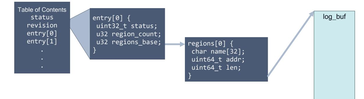
On Qualcomm Technologies devices, firmware traverses the Table of Contents, creates ELF with the regions, and dumps the ELF to storage medium (typically eMMC/UFS/SD card)
