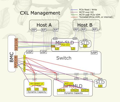
Tunneling between devices is over MCTP over PCIe VDM
