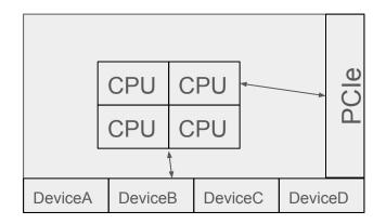
Same SoC, but cores are disabled and connected to host system as a PCIe Endpoint. Already have drivers for DeviceA, DeviceB, etc.
