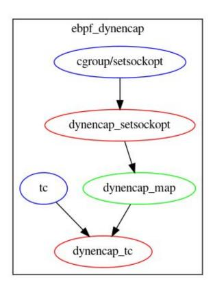
dynencap\_map is an SK\_STORAGE\_MAP that records the IPs to use when encapsulating the packets from a socket.
