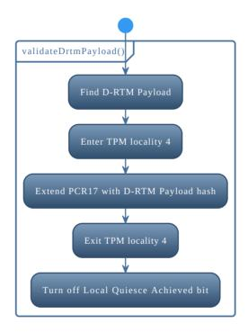
• MPIPL (Memory Preserving Initial Program Loader) - part of OpenPOWER firmware which executes special boot path skipping memory training, ECC initial pattern writing and executes D-RTM Payload, if it was set.
