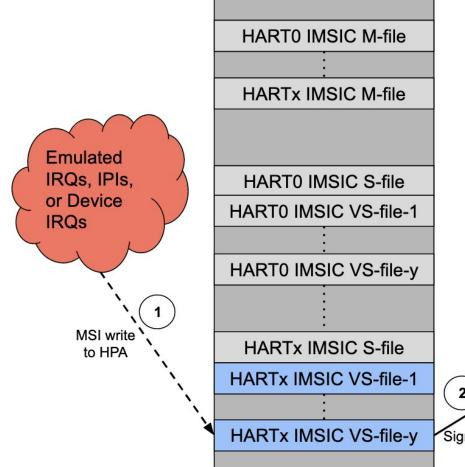
**Example:** Wake-up Guest\_A VCPU\_B from WFI using IMSIC VS-files on HARTx
