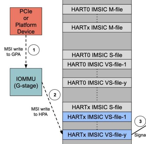
**Example:** MSI from PCIe (or Platform) device targeting Guest\_A VCPU\_B using IMSIC VS-files on HARTx
